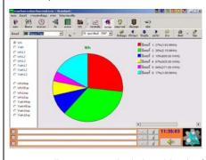
Automatically summaries the kwh and kvarh of all meters compared to overall energy to show ratio or area consumed efficiency.
