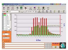
Automatically comparing kwh per hour of each meter to show energy consumption efficiency compare with time.
